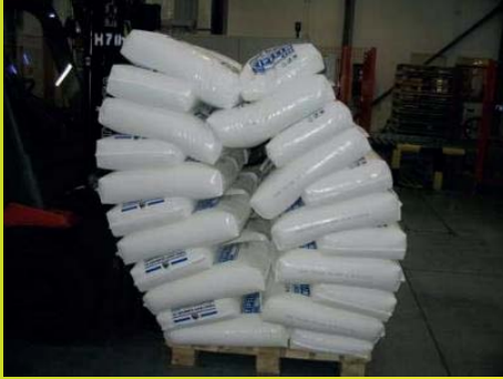
Leaning pallets off shape
