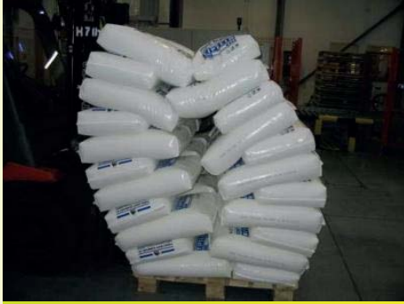
Leaning pallets off shape
